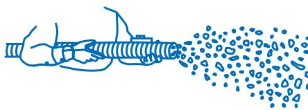
Blow insulation to the desired thickness.
