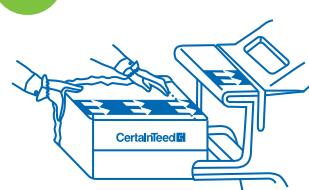
Place 1/2 of the package on the hopper tray by lining up the arrows and cut package.
