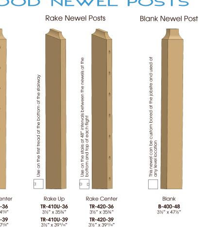
Each newel post includes a ¾" x 2" wood dowel (Dowel) for attaching the 684 Handrail
