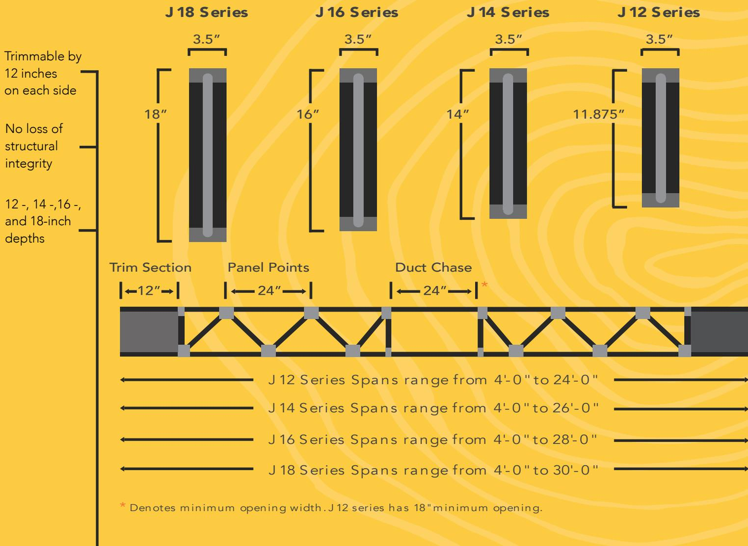
The engineered strength of the TrimJoist<sup>®</sup> system provides for longer spans and wider on-center spacing. Joists come in two-foot incremental lengths, beginning at 4 feet and spanning as far as 30 feet and can be trimmed by up to 24 inches.
