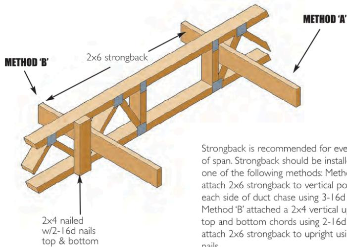
Strongback is recommended for every 10'-0" of span. Strongback should be installed using one of the following methods: Method 'A' attach 2x6 strongback to vertical posts on each side of duct chase using 3-16d nails. Method 'B' attached a 2x4 vertical upright to top and bottom chords using 2-16d nails and attach 2x6 strongback to upright using 3-16d nails.
